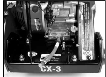
(C) Free the Oil Drain Line. Place a catch basin below the Oil Drain Line. Remove the Drain Cap to drain oil completely. Refer to Engine Manual for details.
