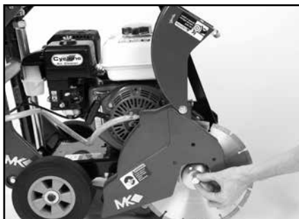
(G) Install the Blade Retaining Bolt.
