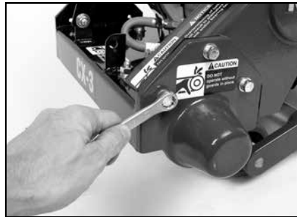
(K) Install the Blade Shaft Cover.
