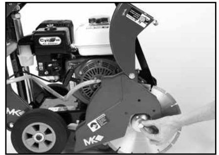
(C) Remove the Blade Retaining Bolt and the Outer Flange.
