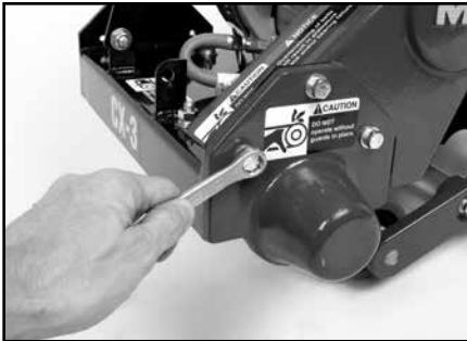
(G) Remove the Blade Shaft Cover Retaining Bolts and the Blade Shaft Cover.
