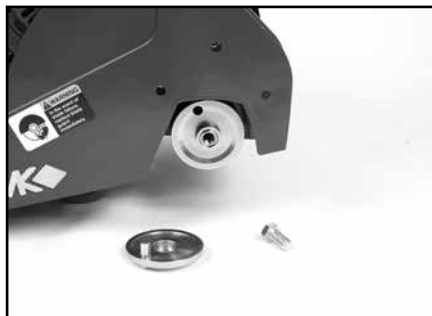
(D) Loosen the Blade Retaining Bolt while holding the Shaft Wrench steady. Remove the Blade Retaining Screw and Outer Flange.
