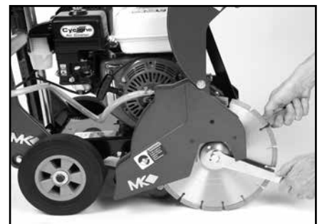
(F) Tighten Blade Retaining Bolt while holding the Blade Shaft steady.
