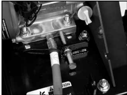
(G) Loosen the Motor Tension Arm. Push the Motor forward to loosen the belt.
