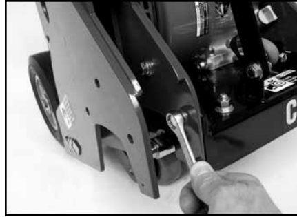
(E) Remove the Blade Guard Retaining Bolts and remove the Blade Guard.
