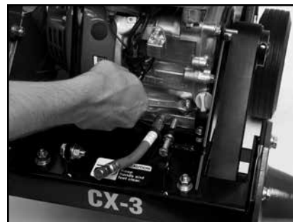
(O) Tighten the Engine Mounting Bolts.
