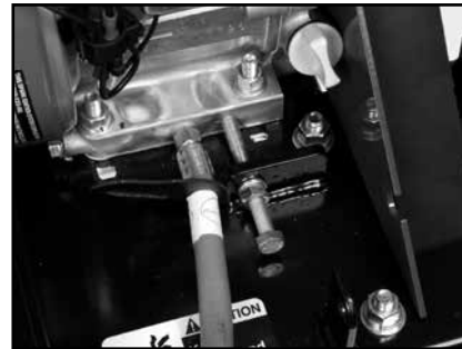
(L) Tighten the Motor Tension Arm.
