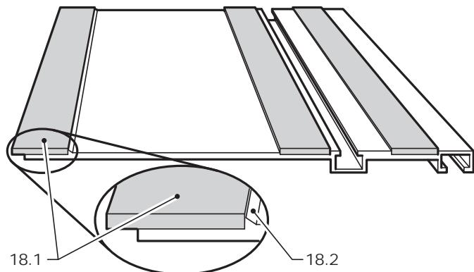
The splinter guard needs to be replaced if it becomes damaged or worn:
