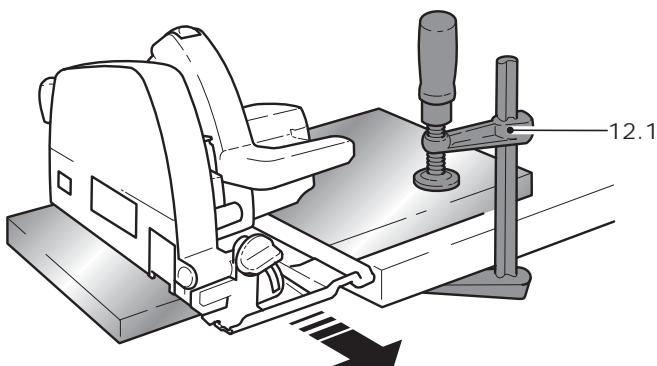
Ensure that your workpieces are securely fixed and cannot move during sawing. Otherwise, there is an increased risk of accident. Never hold the work-piece to be cut with your hands or between your legs. Use instead screw clamps (12.1) or some other suitable devices to fix your workpiece.
