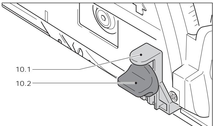
The splinterguard (accessories) significantly improves the quality of the cutting edge of the sawn workpiece on the upper side for 0° cuts.
