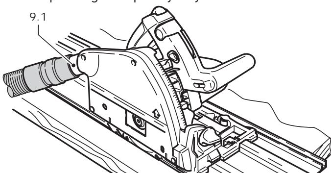
A Festool dust extractor with an extractor hose diameter of 36 mm or 27 mm (36 mm recommended)
