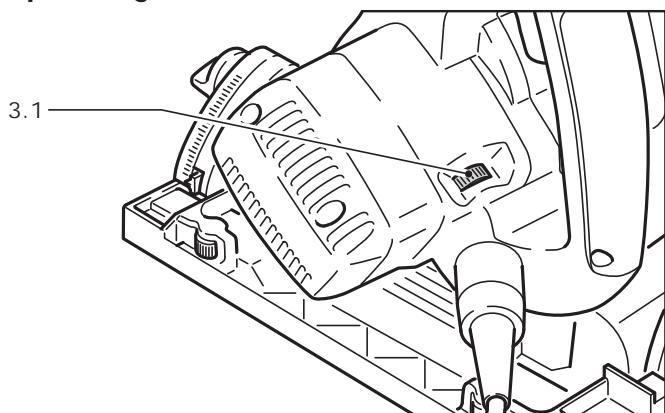
The speed controller (3.1) provides infinitely variable setting between 1350 and 3550 rpm of the speed of the saw blade. This enables you to optimize the cutting speed to suit the material.
