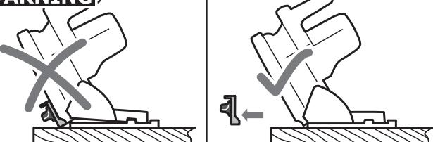
**Use the splinterguard only for 0° cuts. Always remove the splinterguard for mitre cuts.** When making mitre cuts, the splinterguard raises the portable circular saw from the workpiece, which can lead to serious injuries.
